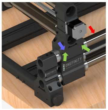
**Step 5:** Once you have ensured the Y-Axis Gantry Blocks and X-Axis Rails Ends are flush, fasten the front of the X-Rail to the Y-Axis using four (4) X-Rail Mounting Screws (Blue Arrows)
