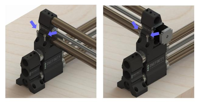
**Step 6:** Fasten the back of the X-Rail to the Y-Axis using the remaining four (4) X-Rail Mounting Screws (Green Arrows)
