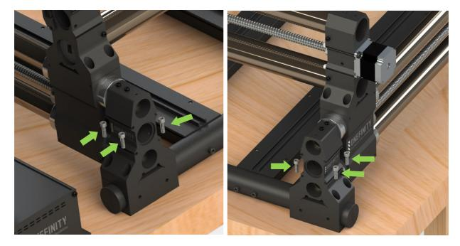
**Step 11:** Repeat steps 14 and 15 to jog the Y-Axis until the X-Rail is to the back of the machine again. Finish fastening the Y-Rails to the QCW Frame using the remaining three (3) Y-Rail Mounting Screws per side (Green Arrows).
