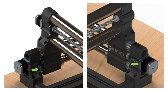
**Step 10:** We will now finish fastening the front Y-Rails. Push the X-Rail all the way to the front again, finish fastening the Y-Rails to the QCW Frame using another three (3) Y-Rail Mounting screws per side (Green Arrow).
