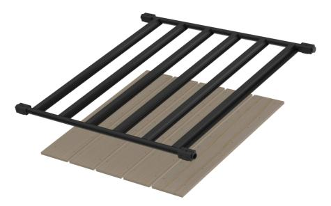
**Step 2:** Ensure the wasteboard is flush with the front of QCW Frame Tube and secure your wasteboard using the suppled screws. **Very Important Note:** Set the torque on your drill to low and finish tightening the screws with a hand screw driver. If your drill torque is set too high the screws may strip!
