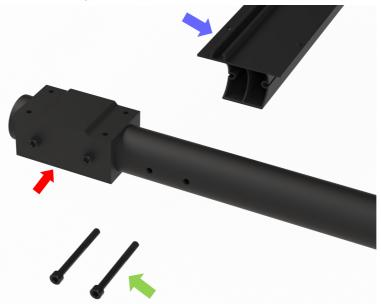
**Step 2:** Attach the rest of the T-Track Extrusions to the QCW Frame Tube Assemblies using the remaining QCW Frame Assembly Bolts. **Note:** To make the assembly process easier, wait until you have all the T-Track Extrusions attached before fully tightening the QCW Frame Assembly Bolts.
