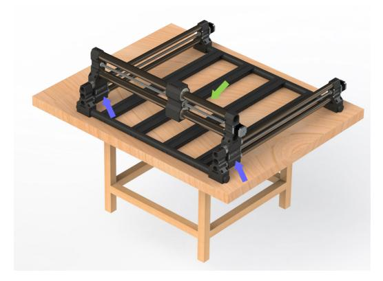
Step 3: Place the X-Rail (Green Arrow) on the Y-Rails Gantry Blocks (Blue Arrows)
