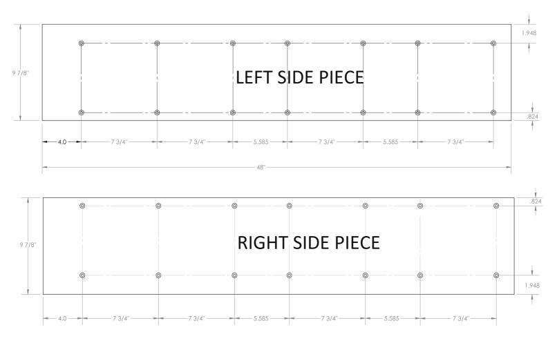
**Step 4:** Insert your Forstner Bit into your drill and counter bore holes in the locations you centre punch in step 3. **Important Note:** Counter bore to a depth of 3/8"
