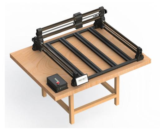
**Step 9:** After moving the X-Axis all the way to the back, fasten the back of the Y-Rails to your QCW Frame using only one (1) Y-Rail Mounting Screw per side (Green Arrow).
