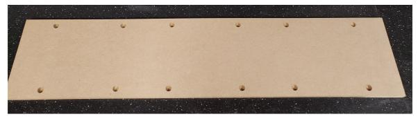
**Step 6:** Using a 1/16" Drill Bit, drill through holes in the centre of the counter bored holes. **Note:** Preforming this step helps to minimize chipping of the MDF.
