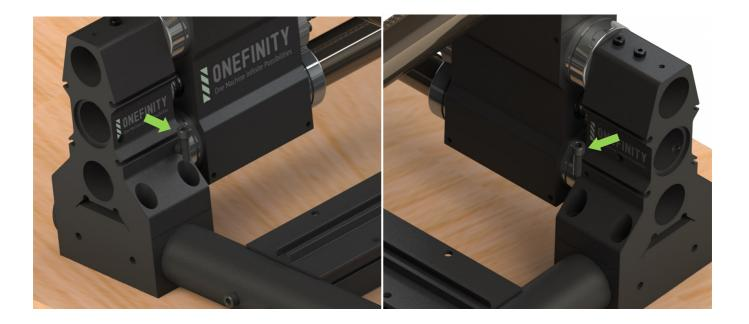
**Step 8:** After fastening the front Y-Rails, push the X-Rail to the back of the machine as shown below.
