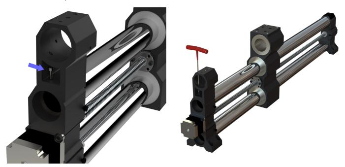
**Step 8:** With the Right Side Stiffy Rail End secured, slide the X-50 Stiffy Linear Rail through the Linear Bearing and into the secured Right Side Stiffy Rail End.
