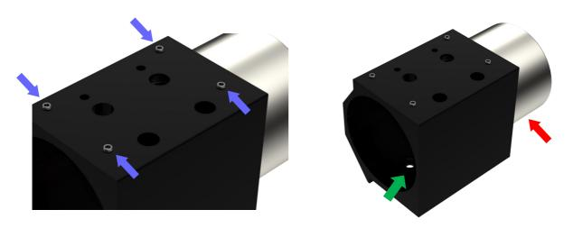
**Step 4:** With the Linear Bearing moved to one side, fasten the Stiffy Gantry Block to the X -Rail using the supplied hardware. Positions the Stiffy Gantry Block so the flat side is facing the Z-Slider. **Important Note:** In this step, use one short screw (Blue Arrow) and one long screw (Red Arrow) The long screw goes closes to the flat side of the gantry Block.
