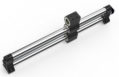
**Step 7:** With the X-50 Stiffy Gantry Block installed, you will now attach the Right Side Stiffy Rail End to the Motor side of the X-50 Rail. Insert the supplied Hex Socket Cap Bolt through the Stiffy Rail End cavity and into the mounting hole (Blue Arrow). With the Hex Socket Cap Bolt inserted into the Mounting Hole, use an Allen Key to tighten the bolt and secure the Stiffy Rail End into place.
