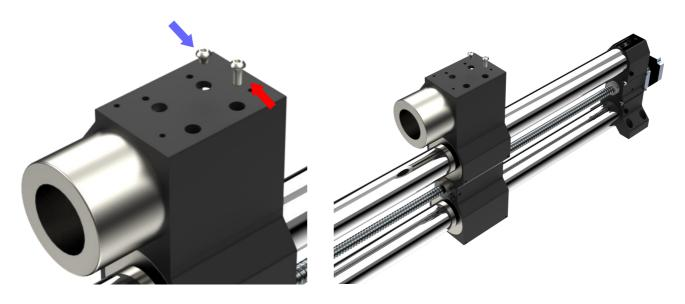
**Step 6:** With the Stiffy Gantry Block secured to the X-Rail Gantry Block, slide the Linear Bearing so it's flash with the Stiffy Gantry Block. Once the Linear Bearing is flush, secure it in place by re-tightening the four (4) Set Screws that you loosened in step 3. (Blue Arrow)
