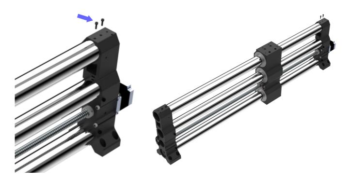
**Step 10:** With the Linear Rail secured to the Rail End, finish securing the Left Side Rail End using the provide Bolt.
