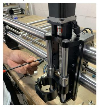
**Step 3:** Square the Z-Slider to your table then tighten the Z-Slider Mounting Screws. Next, plug the Z-Sliders stepper motor into the Curly Cable. **Congratulations, you have finished installed your new Z-20 Heavy Duty Z-Slider!**
