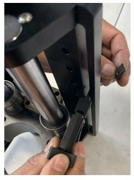
**Step 2:** Repeat the previous step to install the other mounting bracket.
