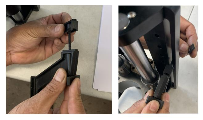
**Step 2:** Repeat the previous step to install the other mounting bracket.
