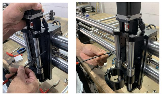
**Step 3:** Square the Z-Slider to your table then tighten the Z-Slider Mounting Screws. Next, plug the Z-Sliders stepper motor into the Curly Cable. **Congratulations, you have finished installed your new Z-20 Heavy Duty Z-Slider!**
