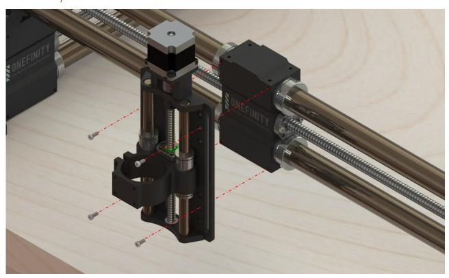
**Step 12:** Square the Z-Slider to your table then tighten the Z-Slider Mounting Screws. Next, plug the Z-Sliders stepper motor into the Curly Cable. **Congratulations, you have finished assembling your new Onefinity CNC Machine!**
