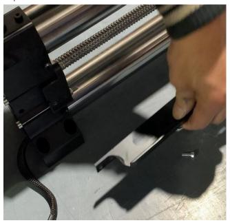
**Step 2:** Remove the Drag Chain Aluminium Extrusion Plastic Bracket using a Hex Key and a wrench. With the Plastic Bracket removed, you can now remove the Mounting Bolts.
