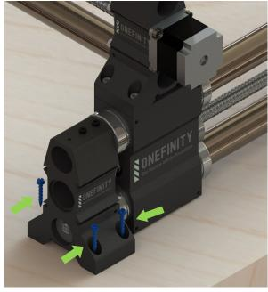
**Step 23:** Repeat steps 19 and 20 to jog the Y-Axis until the X-Rail is to the back of the machine again. Finish fastening the Y-Rails to the table using the remaining three (3) Y-Rail Mounting Screws per side (Green Arrows).
