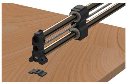
**Step 3:** Place the X-Rail (Green Arrow) on the Y-Rails Gantry Blocks (Blue Arrows)
