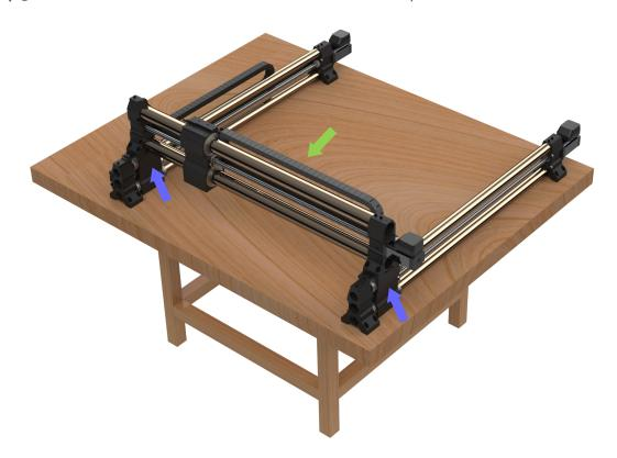
**Step 4:** Adjust Y-Rails (Red Arrows) until the Gantry Assemblies (Green Arrows) are flush with X-Rail Ends (Blue Arrows). **Note:** It is important that these parts are flush with each other before fastening together.
