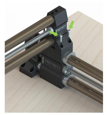
**Step 7:** Fasten the front of the Y-Rails to your table using only one (1) Y-Rail Mounting Screw per side (Green Arrow). You will use the remaining screws later.
