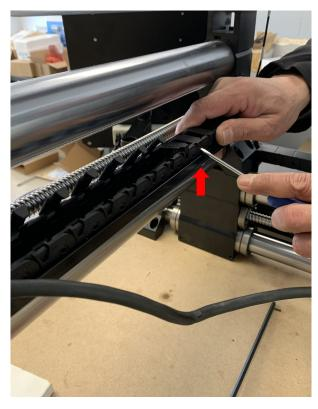
**Step 5:** Insert the Router/Spindle Cable and closed the Drag Chain.
