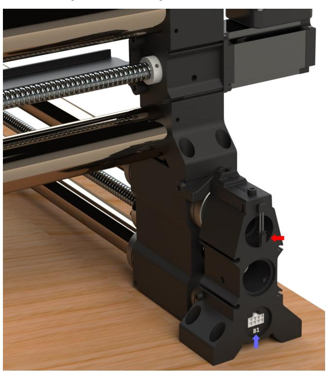
**Step 15:** We'll now connect the Z-20 Z-Slider Wires.
