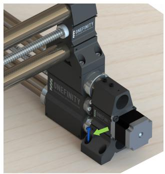
**Step 21:** We will now jog the Y-Axis to bring the X-Rail back to the front of the machine. Press and hold the Y- button (Red Arrow) until the X-Rail is back to the front of the machine.
