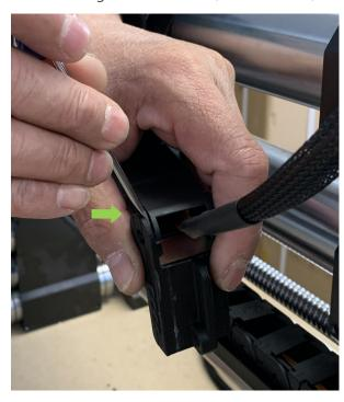
Step 4: Using the small flat head screw driver, open up the Drag Chain (Red Arrow)
