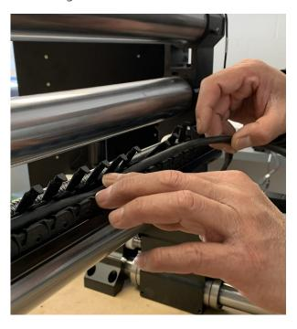
**Step 6:** With the Router/Spindle Cable installed into the Drag Chain, re-connect the Drag Chain Mount to the Drag Chain. Once the Drag Chain and Drag Chain Mount are reconnected, re-attach the Drag Chain Mount to the Gantry Block.
