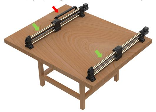
**Step 2:** Slide the Gantry assembly (Green Arrow) all the way to the front until it's tight to the Rail End (Blue Arrow). See below pictures. (Note: you can also turn the ball screw to get the Gantry Assembly to move to the front). **Important:** Make sure they are all the way to the front!
