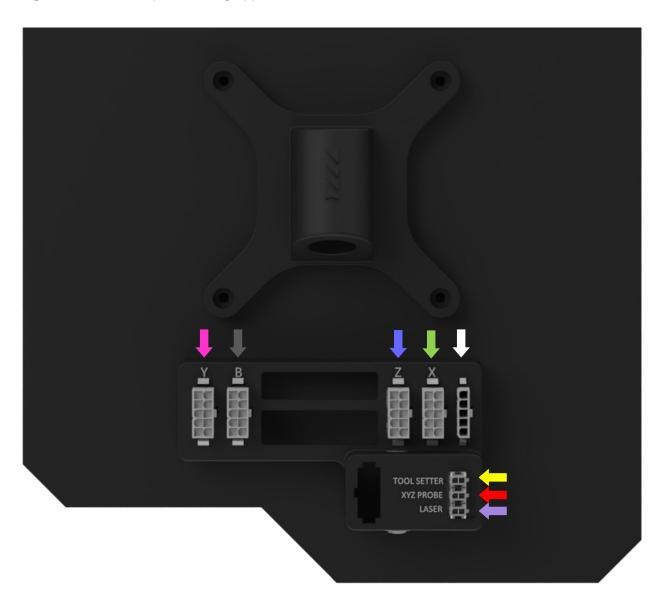
**Step 17:** We'll now connect the Power Supply Controller Wires.
