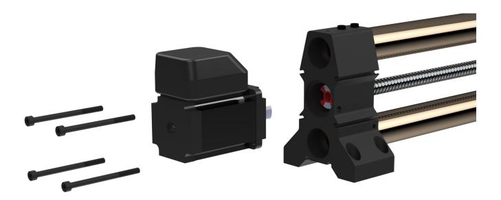
We are now going to connect the Stepper Motor wires. Start by removing the Plastic Motor Cover. With the Cover removed, plug in the Wire Connectors to the corresponding connector ports. With the wires now connected, re-install the Plastic Motor Cover. **Important:** Pay attention to how the wires exit the cover. See below.
