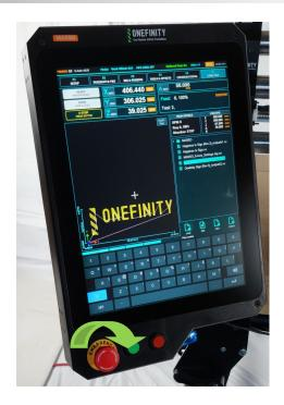
**Step 19:** We will now jog the Y-Axis so we can finish fastening the Y-Rails to the table. First ensure you are on the F<sub>3</sub> page (Green Arrow). Next, press the Continuous Mode button (Pink Arrow). Now, press and hold the Y+ button (Yellow Arrow) until the X-Rail is almost all the way to the back of the machine. **Note:** If you find that it's jogging to slow you can increase the Feed by sliding the Feed bar up (Red Arrow)
