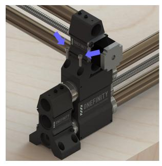
**Step 6:** Fasten the back of the X-Rail to the Y-Axis using the remaining four (4) X-Rail Mounting Screws (Green Arrows)
