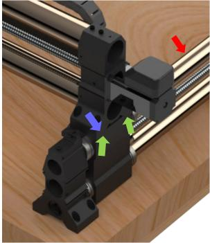
**Step 5:** Once you have ensured the Y-Axis Gantry Blocks and X-Axis Rails Ends are flush, fasten the front of the X-Rail to the Y-Axis using four (4) X-Rail Mounting Screws (Blue Arrows)
