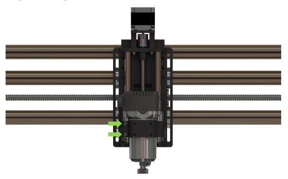
**Step 2:** Unscrew the Cable Clamp and install the router cable (Red Arrow). Disconnect the Z-Axis Stepper Motor and Homing Switch Wires to prevent damage.
