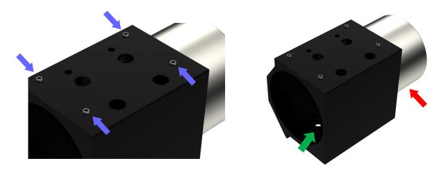
**Step 4:** With the Linear Bearing moved to one side, fasten the Stiffy Gantry Block to the X -Rail using the supplied hardware. Positions the Stiffy Gantry Block so the flat side is facing the Z-Slider. **Important Note:** In this step, use one short screw (Blue Arrow) and one long screw (Red Arrow) The long screw goes closes to the flat side of the gantry Block.
