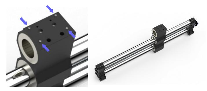
**Step 7:** With the X-50 Stiffy Gantry Block installed, you will now attach the Right Side Stiffy Rail End to the Motor side of the X-50 Rail. Insert the supplied Hex Socket Cap Bolt through the Stiffy Rail End cavity and into the mounting hole (Blue Arrow). With the Hex Socket Cap Bolt inserted into the Mounting Hole, use an Allen Key to tighten the bolt and secure the Stiffy Rail End into place.
