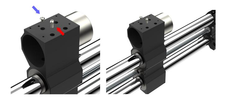
**Step 5:** With the Stiffy Gantry Block secured on one side, slide the Linear Bearing to the other side. Finish securing the Stiffy Gantry Block to the X-Rail using the remain bolts. **Important Note:** In this step, use one short screw (Blue Arrow) and one long screw (Red Arrow). The long screw goes closes to the flat side of the gantry Block.
