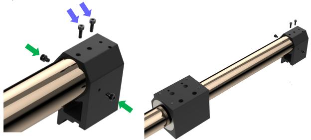
**Step 2:** After removing the top two (2) Stiffy Rail End bolts and loosened the two (2) side bolts, remove the Stiffy Rail End and Stiffy Gantry Block from the Linear Rail.
