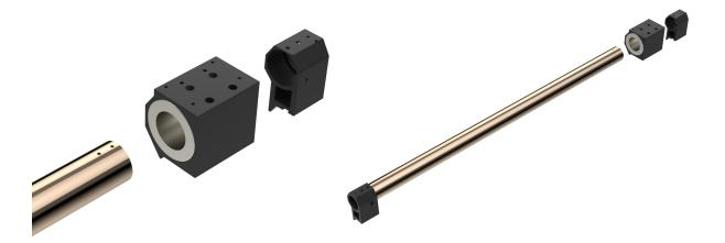
**Step 3:** With the Stiffy Gantry Block removed from the Linear Rail, loosen the four (4) Linear Bearing Set Screws (Blue Arrows). With the Linear Bearing Set Screws Lose, slide the Linear Bearing (Red Arrow) out of the Stiffy Gantry Block until the two (2) mounting holes are visible. (Green Arrow). **Note:** You may need to tap the Linear Bearing with a rubber mallet. **Important Note:** Do not completely remove the Linear Bearing from the Gantry Block.
