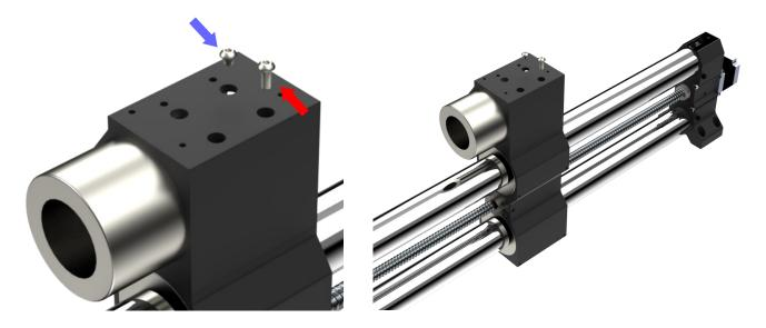
**Step 6:** With the Stiffy Gantry Block secured to the X-Rail Gantry Block, slide the Linear Bearing so it's flash with the Stiffy Gantry Block. Once the Linear Bearing is flush, secure it in place by re-tightening the four (4) Set Screws that you loosened in step 3. (Blue Arrow)
