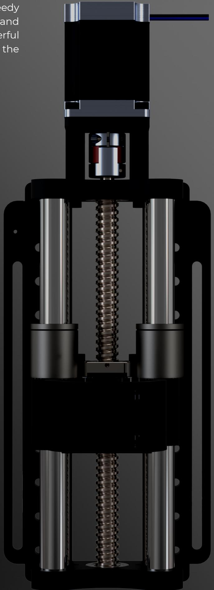
**\*Important Note:** Due to the weight of 80mm Spindles, there is the possibility that the Z-Axis may drop when powering down or using the Emergency Stop. This may be amplified when adding a Spindle Mounted Dust Shoe.
